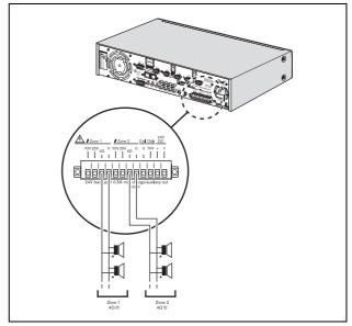
figure 4.9: Connecting speakers
